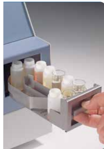
3. After the analysis is run, the used sample is collected in the discharger tray.
