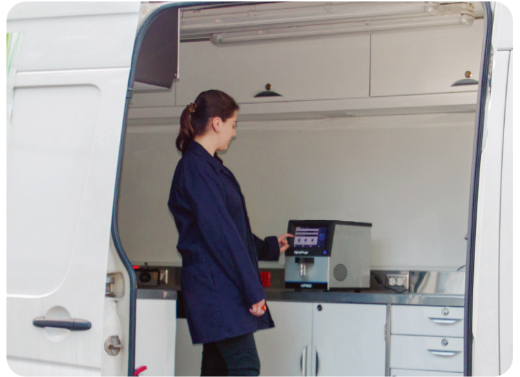
Mobile Lab is enclosed climate controlled lab with ambient temperature and humidity within product specification to obtain desired performance.
